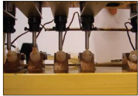
Fig. 1. Left: A specimen placed in the fatigue tester at a 45 degree angle for cycling. Right: A fatigue tester with the five stations for cycling.
