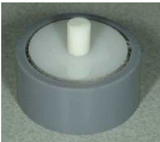
Fig. 1 The Y-TZP disc specimen was embedded in the PMMA with the cementation surface exposed. Cement was applied incrementally, not exceeding 2 mm, to the surface using polyethylene molds (inner diameter=3.6 mm, height=5 mm) and polymerized accordingly
